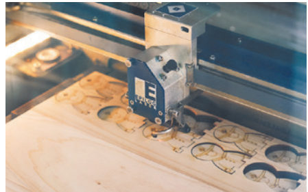
Laser cutting of Copper Mine Building Blocks
