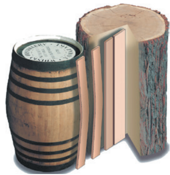
How timber is taken from logs to make barrels
