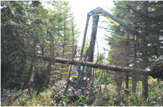
Integrated operations with a harvester (felling, debranching, processing)
